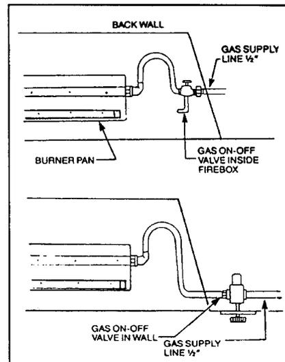
**Figure 3 - Gas line installation
